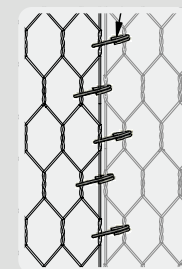
Raccordement sans recouvrement
